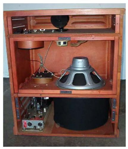
In this picture of a Leslie speaker with the back removed, you can see the rotating drum below the bass speaker unit.
